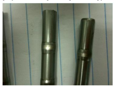
liner turning it into an abrasive surface that can in some cases cause premature valve stem wear.
